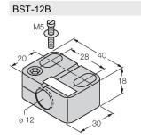
6947212 Mounting clamp for threaded barrel sensors, with dead-stop; material: PA6
