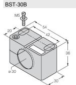
6947216 Mounting clamp for threaded barrel sensors, with dead-stop; material: PA6
