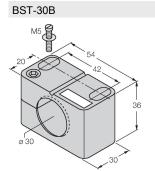
Mounting clamp for threaded barrel sensors, with dead-stop; material: PA6
